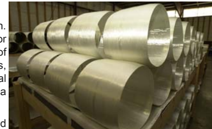
Forming cakes, or rolls, of fiberglass yarn will be woven into fabric at Dielectric Solutions.
